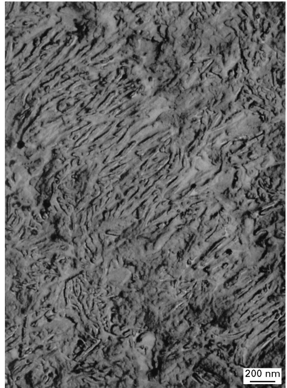
Figure 8 Lamella stack oriented perpendicularly to weld line (PE-HD3) (TEM, 25 000×, tilt 0°).
