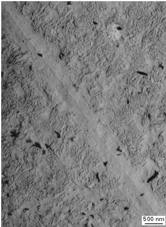
Figure 7 The weld line area of PE-HD3 (TEM, 12 000×, tilt 0°).
